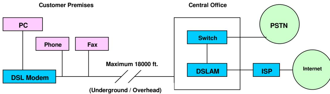
DSL Modem or DSL Transceiver, as it is also referred to as, is connected to the customer's computer via USB or a 10-Base T connection.
